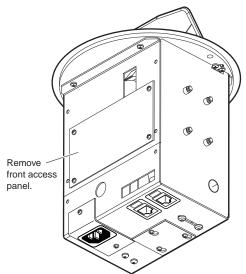
Figure 3-1 — Removing the front access panel (HSA 222 models)
